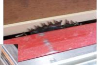
the top moves in, it will leave saw marks. Cut all 4 sides, rolling the box toward you. Now you have to finish cutting the top loose with a hand
