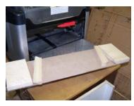
Because I make a lot of these boxes, I decided to make an adjustable sled for the front/back and ends. Use a <sup>1</sup>/<sub>4</sub>" hard board base and glue 4" x 7" blocks 18" apart. Cut 1" x 7" blocks that can be taped in place for the 16" pieces.
